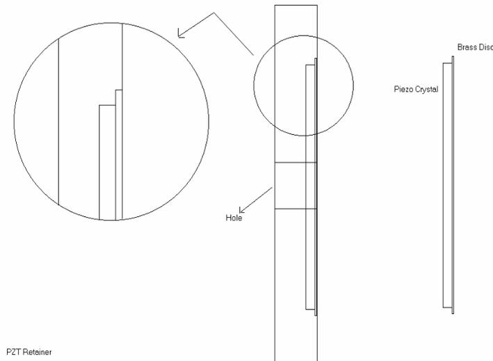
Figure 2: Diagram showing the PZT and Mount
