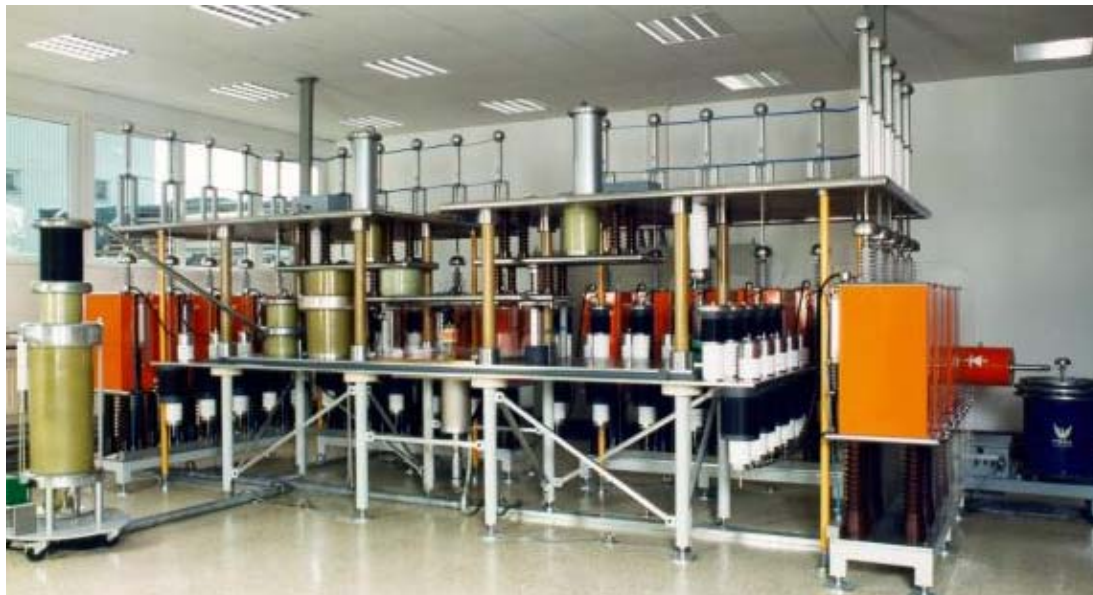
Fig. 9 Crow bar generator for 10/350 \mu s wave shape, 200 kA peak current, 100 As charge transfer and 10 MJ/Ohm specific energy.
