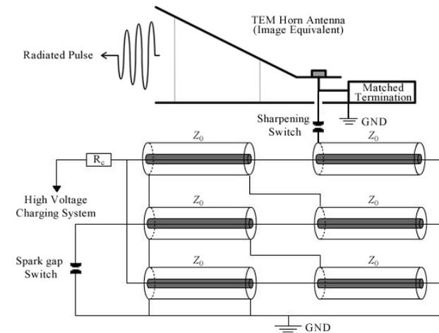
Figure 1. Schematic layout of EMI Generator
