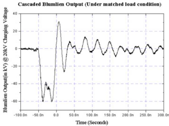
**Figure 2.** Oscillogram of Output Voltage before pulse sharpening, when pulser is charged up to 20kV
