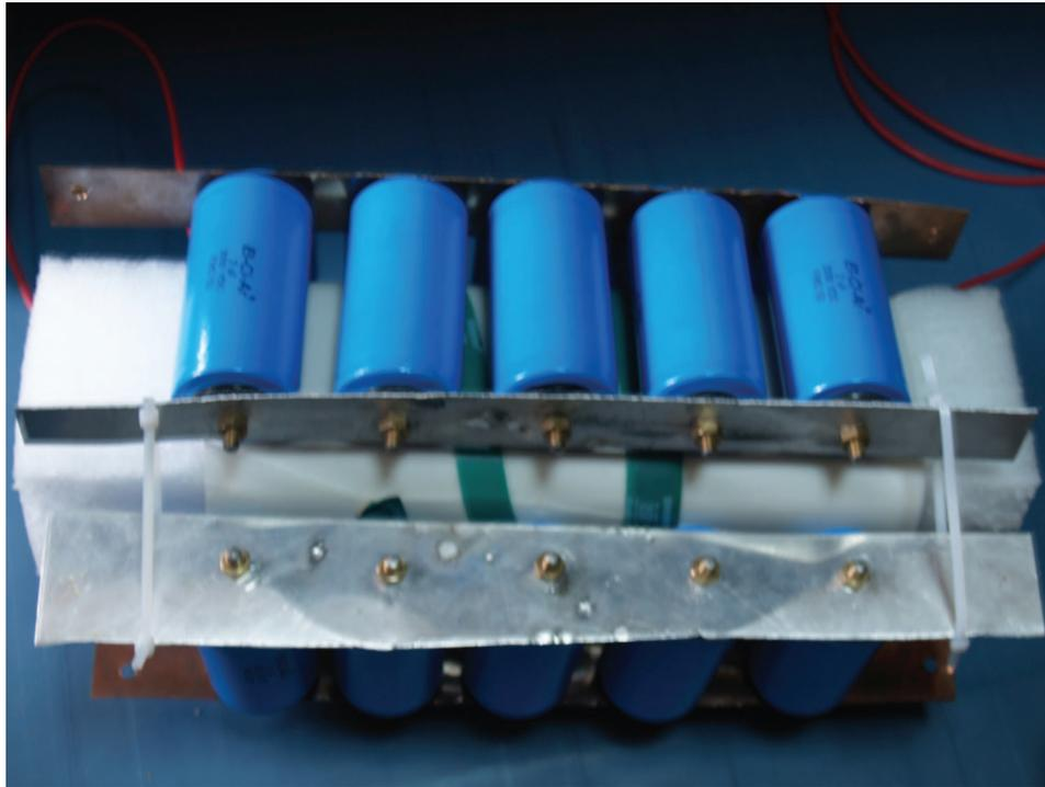
FIG. 1. (Color online) Compact pulse transformer using capacitor bank as its primary.
