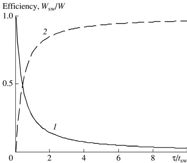
Fig. 6. (1) Switching-off loss and (2) efficiency versus  $\tau/t_{sw}$ .
