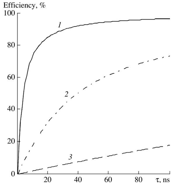
**Fig. 5.** Efficiency versus circuit time constant for  $t_{sw} =$  (1) 10 ns; (2) 100 ns; and (3) 1  $\mu$ s.
