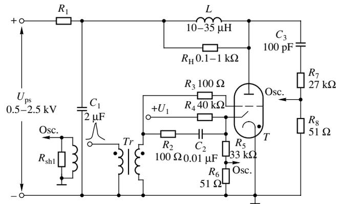
**Fig. 2.** Experimental-setup circuit diagram.
