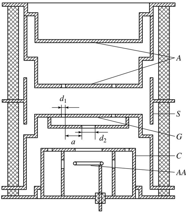
**Fig. 1.** Design of the pseudospark-gap under investigation: (A) anode; (S) protective screen; (G) control grid; (C) cathode; (AA) auxiliary anode; ( $d_1$ ) diameter of the grid openings; ( $d_2$ ) diameter of the grid-screen opening; and ( $a$ ) overlap of the grid openings and the grid-screen opening.
