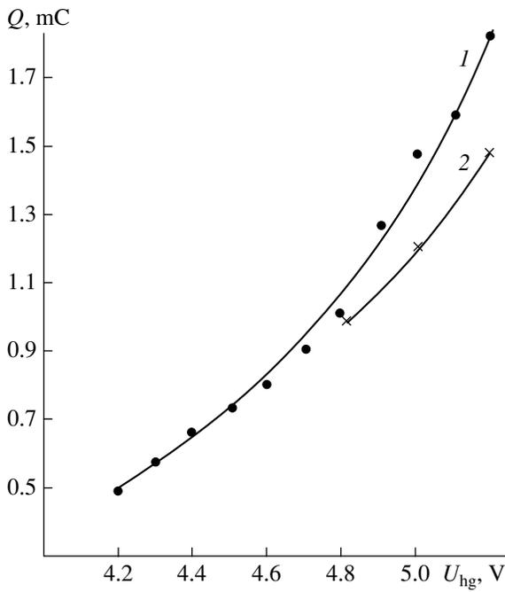
**Fig. 3.** Charge required for current interruption in (1) ТТН2-500/20 thyatron and (2) PSG versus hydrogen-generator filament voltage  $U_{hg}$ .
