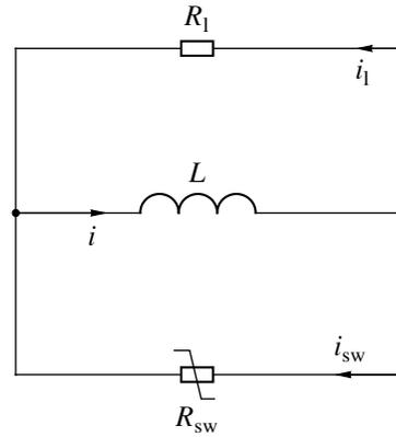
**Fig. 4.** Simplified circuit diagram of the high-voltage part of the generator for the moment of current interruption.
