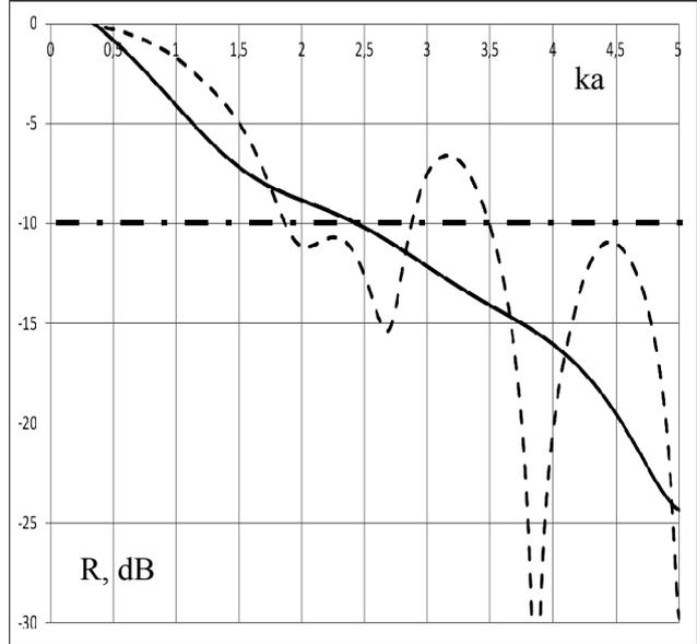
Fig. 5. The dependence of the reflection coefficient on the electric size of the sphere (formula (3),  $n = 4$ )
