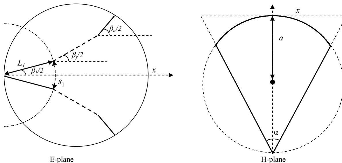
Fig. 1. A piece-wise linear TEM-horn.
